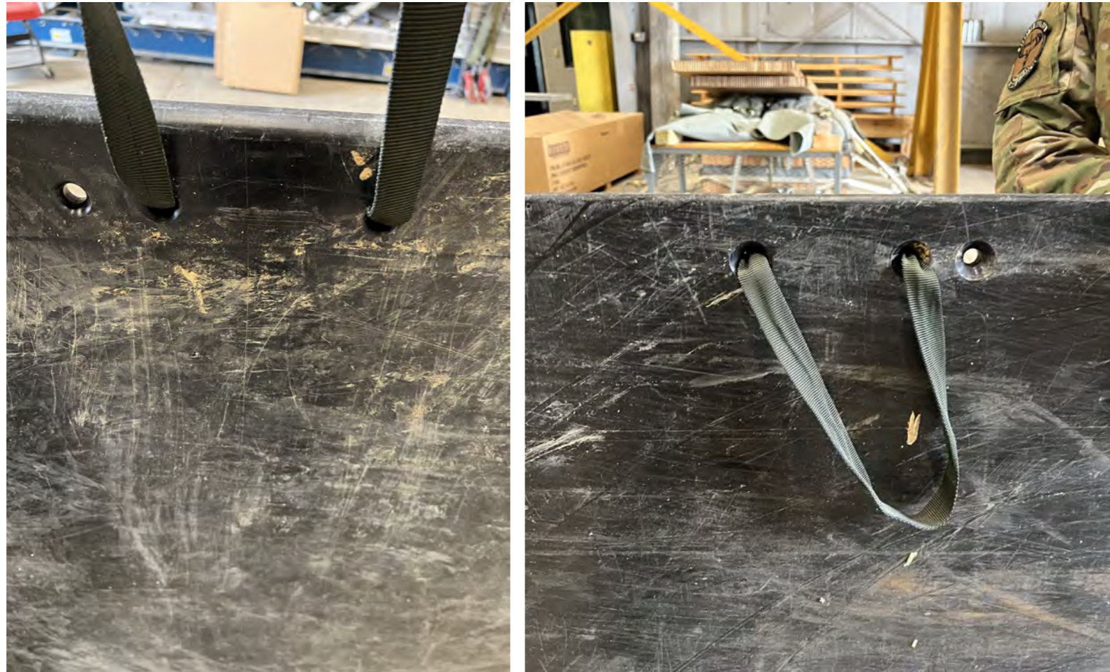
Front and Back of RUSB after pull test
