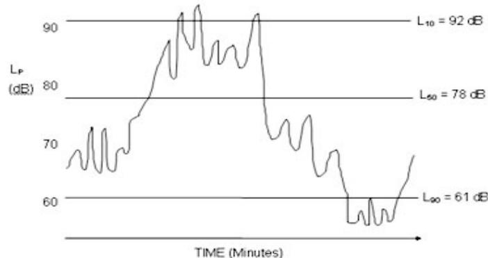
L<sub>10</sub> is the noise level exceeded for 10% of the time of the measurement duration. This is often used to give an indication of the upper limit of fluctuating noise, such as that from road traffic.
